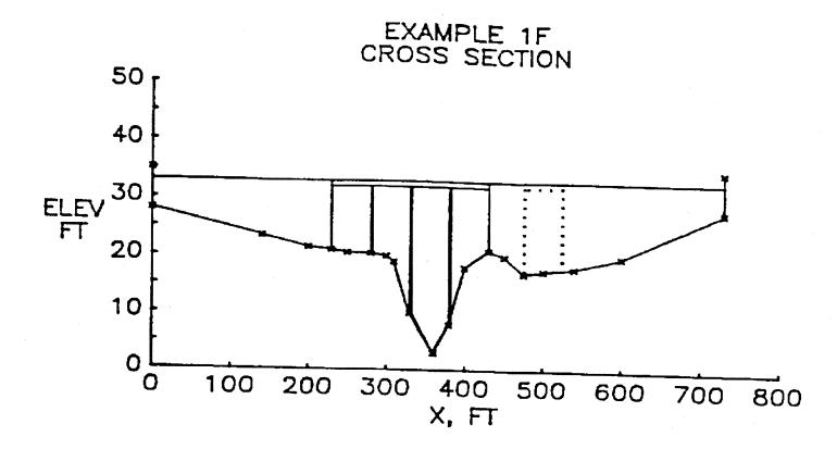
Figure B.9 Backwater For Multiple vs. Single Bridge Opening
