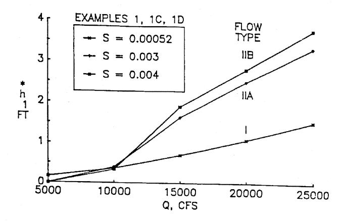
Figure B.5 Bridge Velocity For Flow Types I, IIA, IIB
