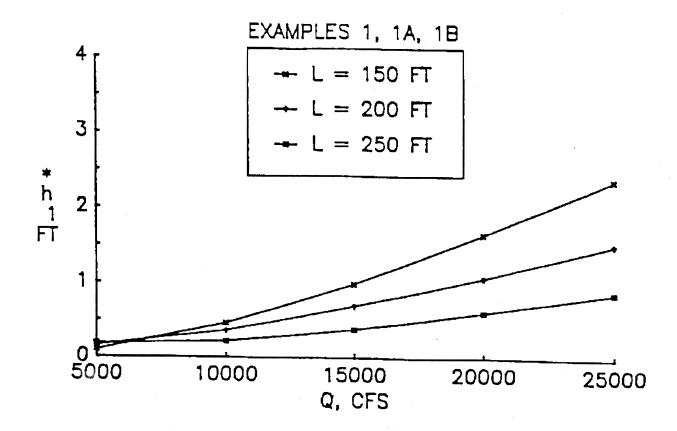
Figure B.3 Bridge Velocity For Examples 1, 1A, 1B With Varying Bridge Opening Length L
