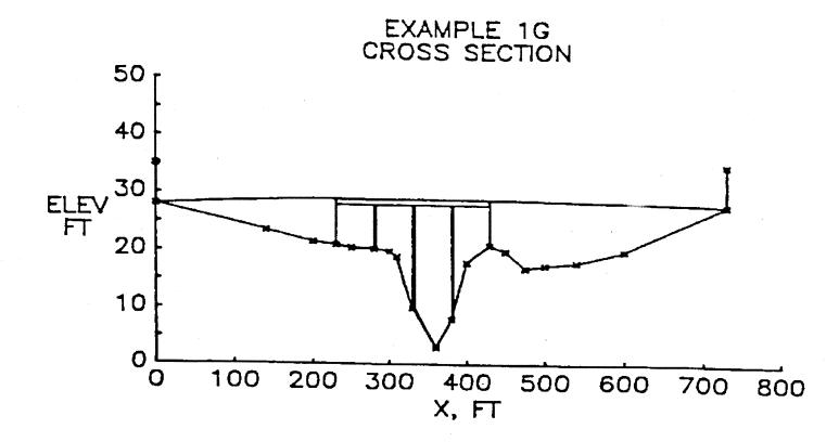
Figure B.11 Backwater Effects Of Embankment Overtopping
